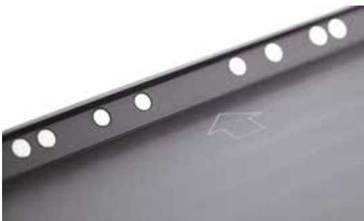
magnets holding the iPad
